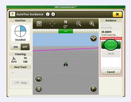
Select "Set B." Once hitting this, system will snap a line directly between Point A and Point B.
